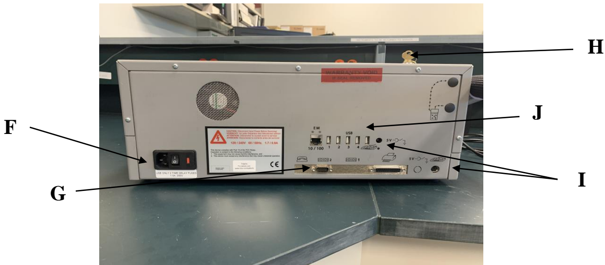
Figure 2. Intoximeter EC/IR II Rear Panel Connectors and Controls
