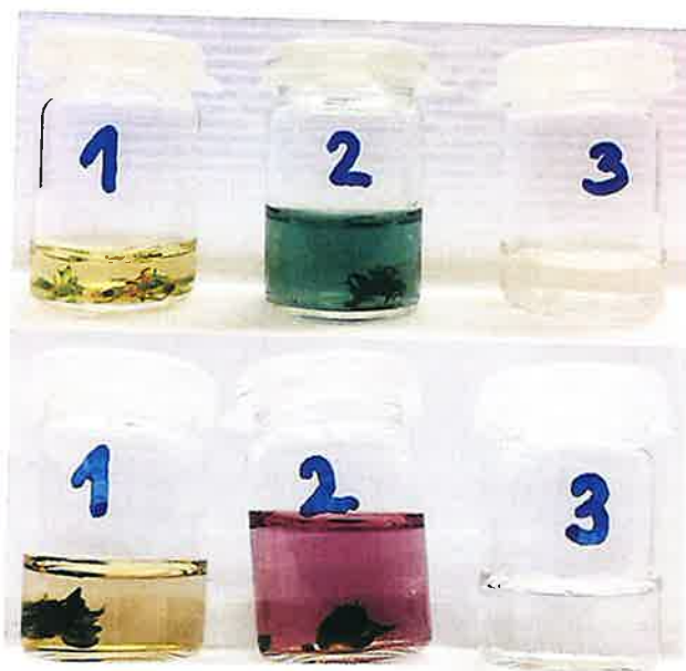
Fig. 1 Colorimetric on-site test (vial 1: cannabis sample with solution 1; vial 2: cannabis sample with solutions 1 + 2; vial 3: solution 1 as reference). Blue coloration (center top) indicates THC-rich cannabis; pink coloration (center bottom) indicates CBD-rich cannabis
