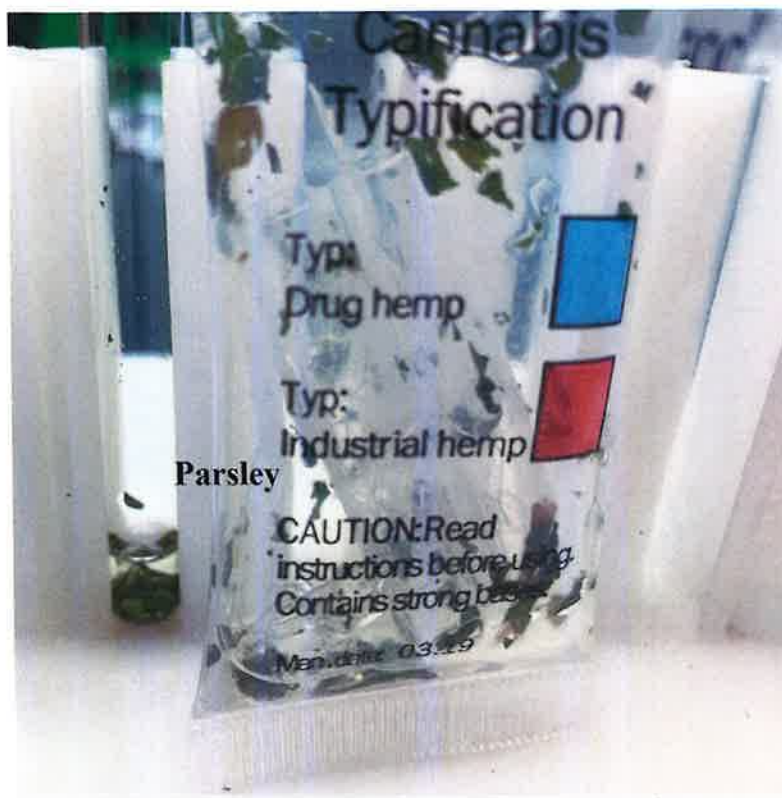
Parsley run with 4-AP color test and field test kit
