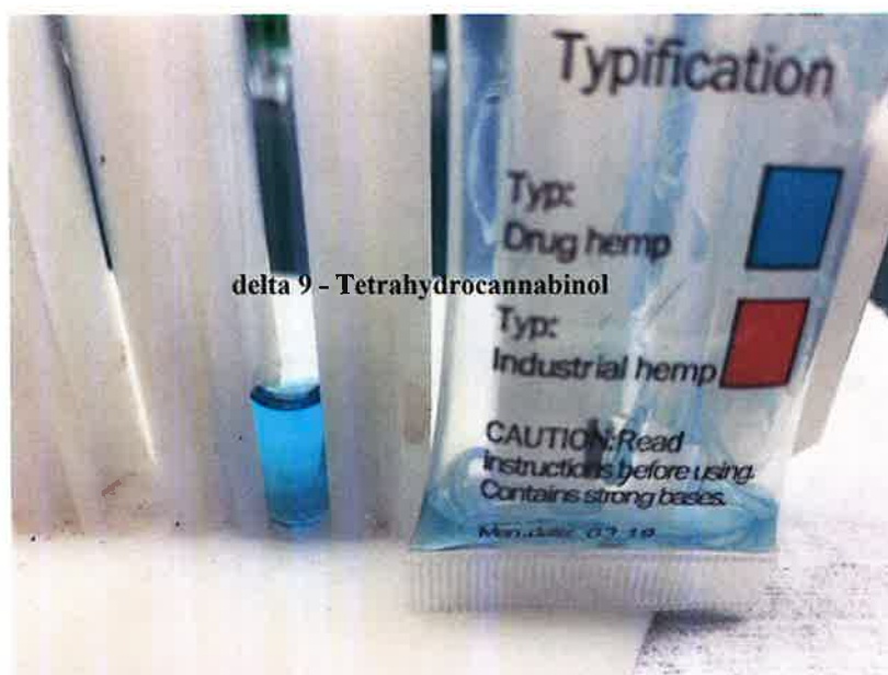
\Delta^9 -Tetrahydrocannabinol Standard with 4-AP color test and field test kit
